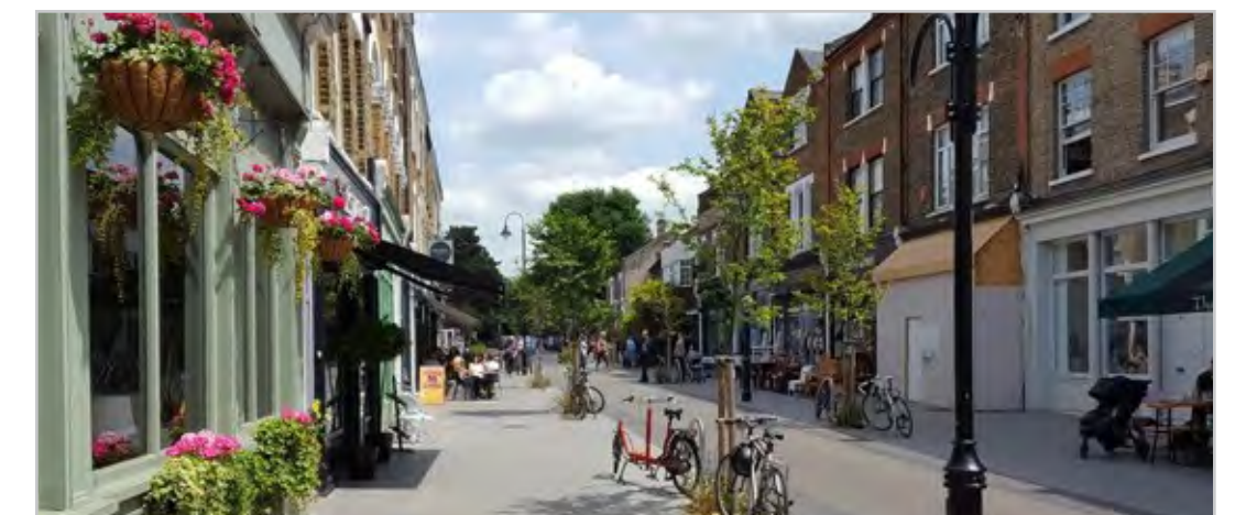
Orford Road, Walthamstow Village – Footway widening, cycle parking stands and one-way traffic flow with time restrictions on motorised traffic (except buses)
