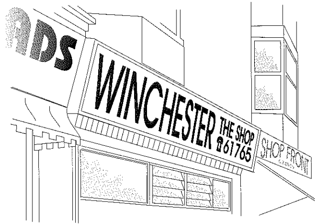
An unacceptable illuminated fascia box sign. Which is crude and over dominant, obscuring fascia detail and dark lettering on light background.
