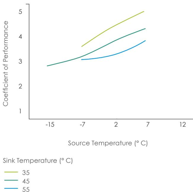
**Figure 3.2** - Typical manufacturer test data for an 8kW air source heat pump showing efficiency at different source and sink temperatures.
