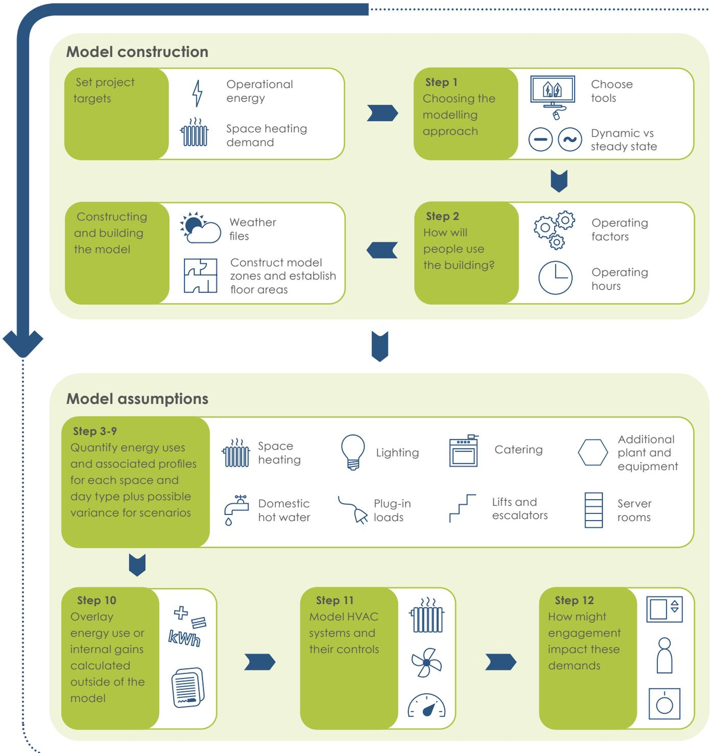
Figure 2.10 - TM54 modelling process
