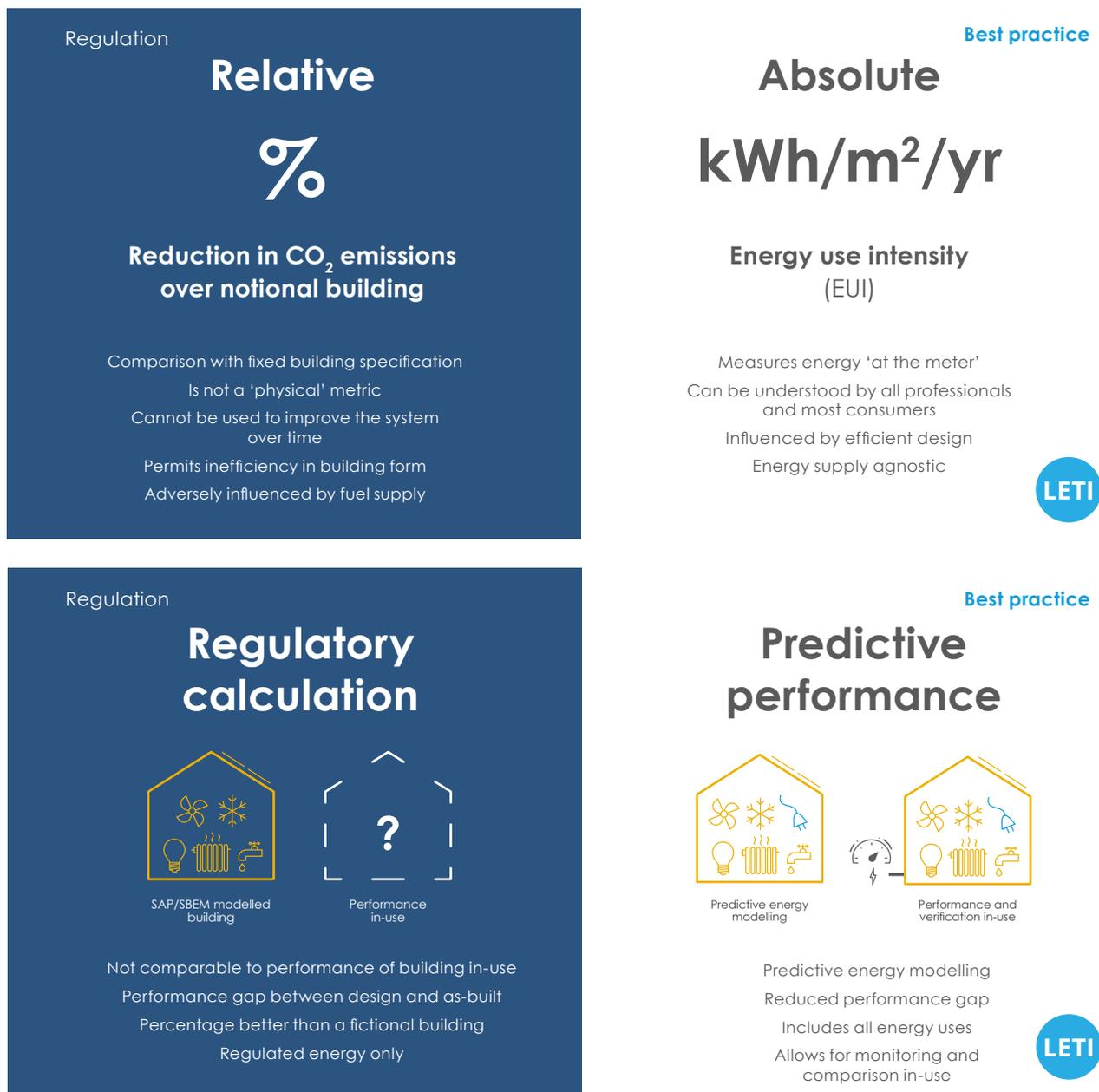
Figure A1.1- The differences between Part L compliance modelling and energy performance modelling
