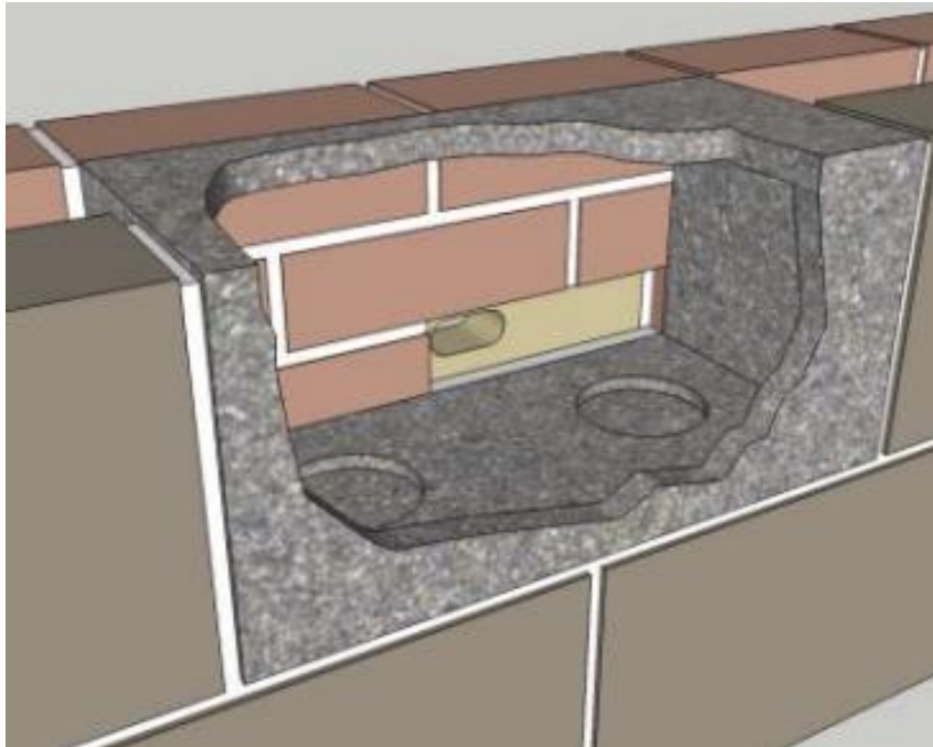
Figure 17. A schematic of how the Cambridge full face Swift brick leads into a cavity created by the prior installation of the Swift maxi nesting box.
