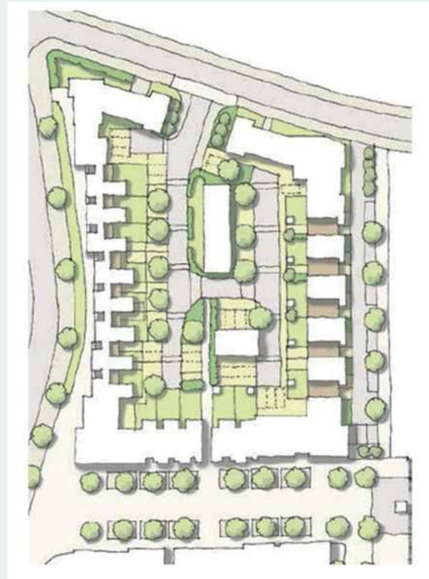
This is a good example of a perimeter block. It has continuous frontages, which address the street. The parking is accommodated within the block, in order to minimise its impact on the public realm. The parking has also been broken up effectively with planting.
