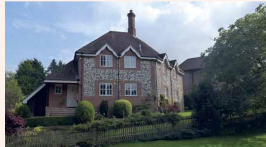
This example in Avington successfully addresses two frontages through the form of the building and the fenestration. This has been individually designed to address the corner, as opposed to using a standard plan form.
