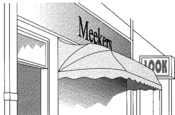
An inappropriate 'Dutch blind'
